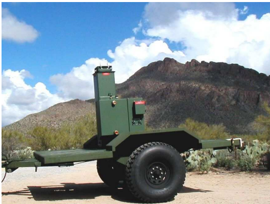
Single mount system with tank and controls mounted on mast.
