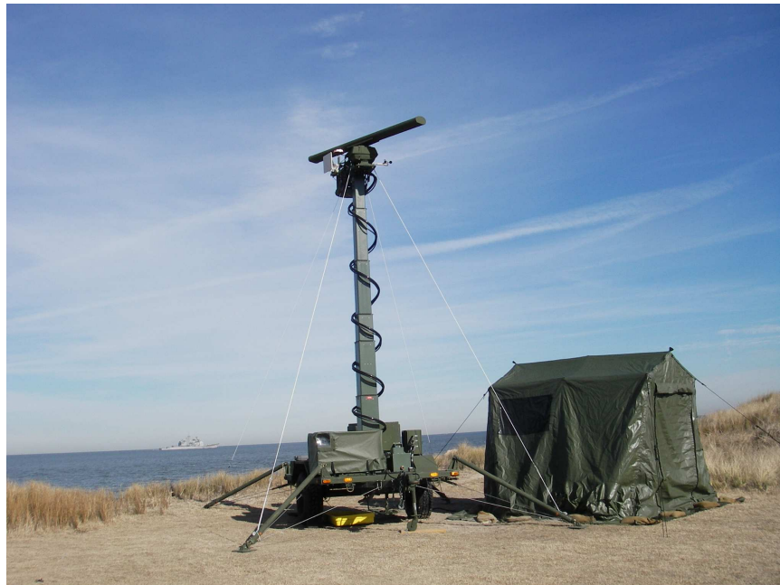
Talon mast system on military tactical trailer deployed with military surveillance systems installed.
