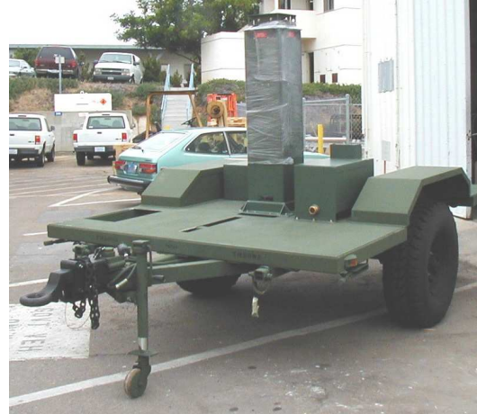
Modular mount system with tank and controls deck mounted.
