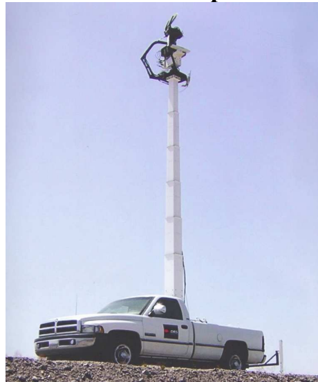
Talon mast system on ¾ ton truck deployed with DRS Technologies sensor suite.
