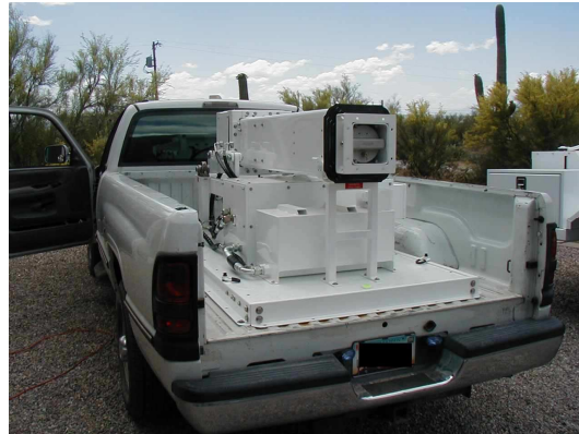
Skid unit mounted in back of truck with truck electrical system Adaptor.
