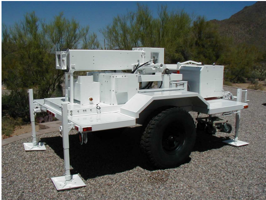
Skid unit mounted on Military Tactical Trailer (LTTFE) With 7 KW generator.
